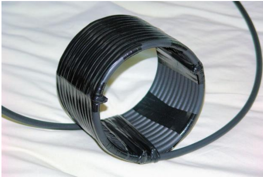
RF choke made with 8-10 turns of feedline coax
