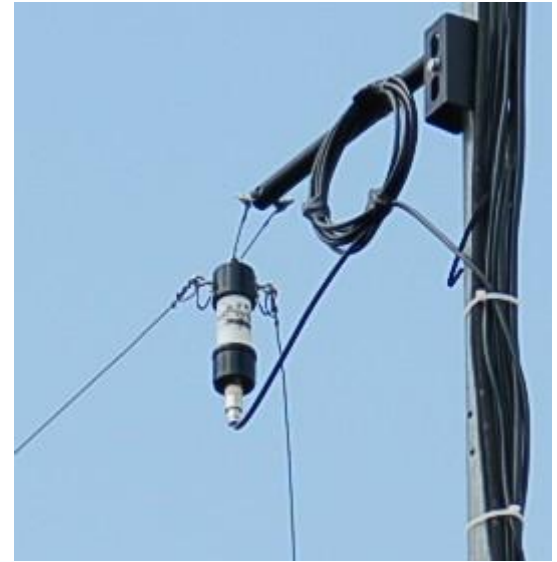
Example of the coaxial feedline choke then feeding the balun
