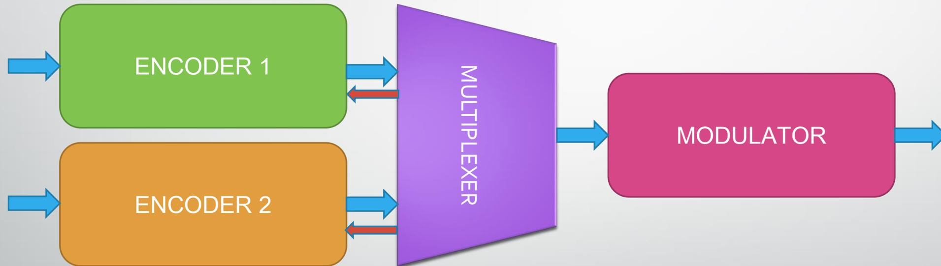
A statmux process is used to create Variable Bit Rate (VBR) encoding
