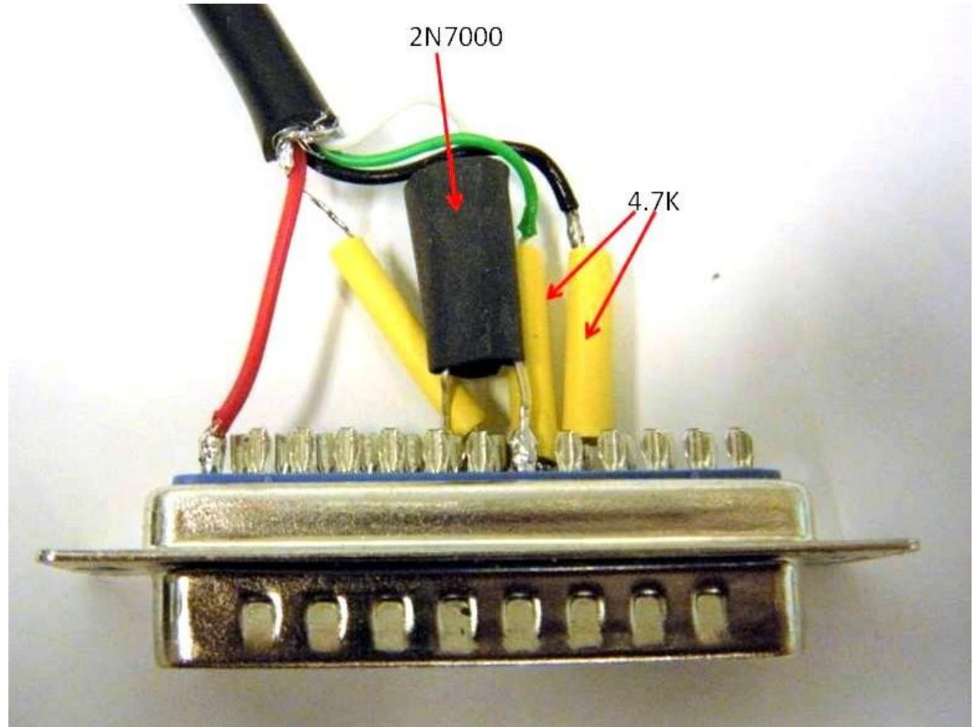
Here is the pinout diagram of the DB25 connector. The source pin of the 2N7000 goes to ground, the drain goes to the COS pin 8, and the gate goes back to the radio to the 10K resistor.
