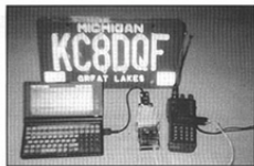
The complete palm-top packet station is smaller than my license plate! From left to right, my HP-200LX palm-top computer, BP-2 modem and HTX-202 transceiver.
