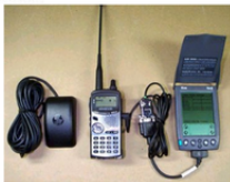
The complete palm-top packet station is smaller than my license plate! From left to right, my HP-200LX palm-top computer, BP-2 modem and HTX-202 transceiver.
