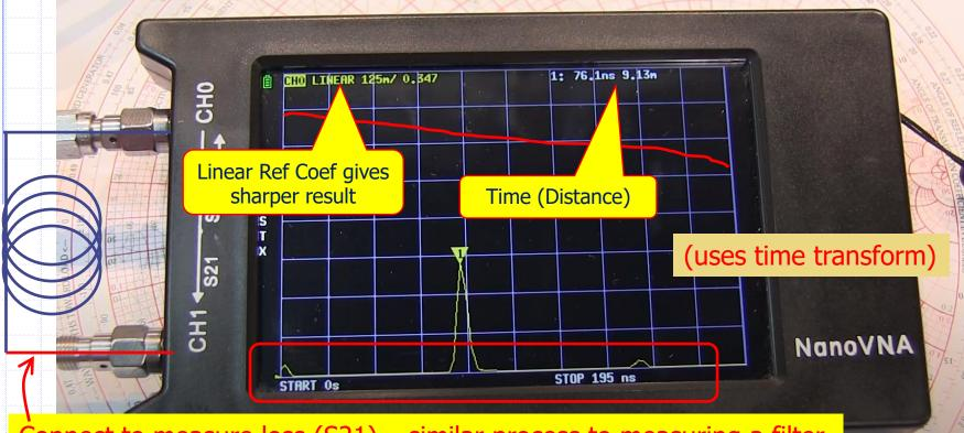
Connect to measure loss (S21) – similar process to measuring a filter
