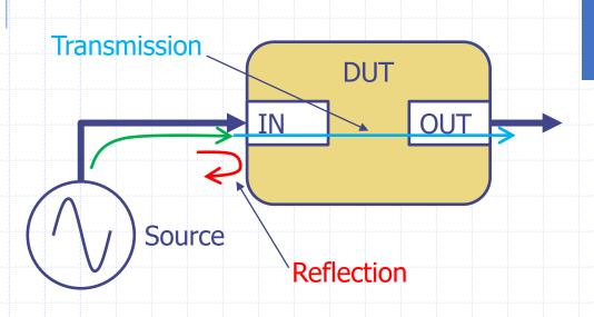
DUT reflection and transmission alter the magnitude & phase of the source signal
